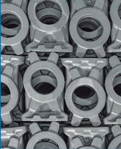
Valve bodies and valve parts are ready just one step before the final assembly of the valve. Just ready to fit our customers' requirements on an extensive range of diaphragm valves, knife gate valves, check valves and penstock valves.
