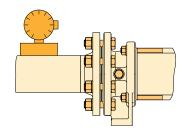
Overpressure protection with bypass and safety valve If the process requires a continuous feed flow and cannot be switched off during operation.
